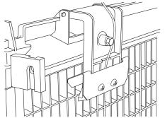
Bridge Thickness Adjustment Mechanism
